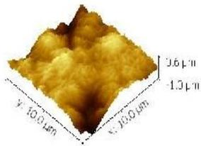
**Figure 3.** 3D view of cdzns Thin Film
