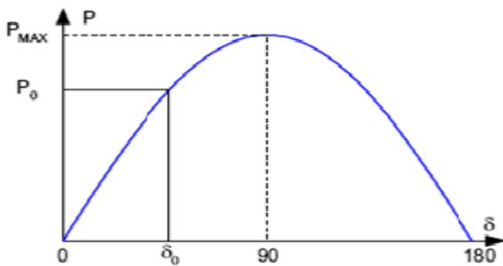
Figure 2. Power Angle Curve
