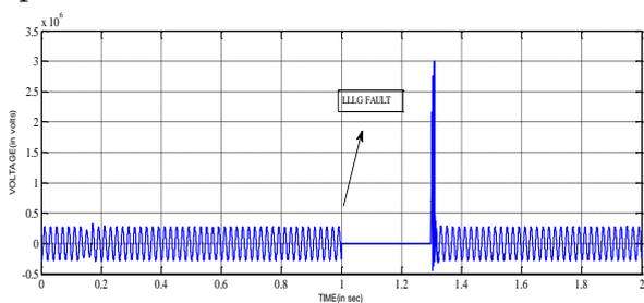
**Figure 16.** Plot of Voltage during three phases to ground fault condition
