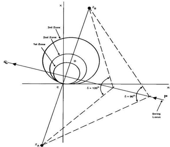
**Figure 6.** Impedance Locus when Line Impedance is small
