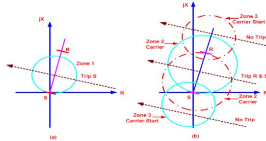
Figure 3. (a) & (b) Zone 1 and Directional Comparison Blocking Scheme Characteristics
