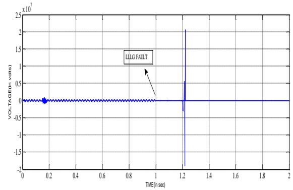
**Figure 20.** Plot of Voltage during three phases to ground fault condition with out OST
