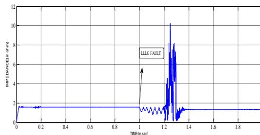
**Figure 17.** Plot of impedance during three phases to ground fault condition without OST
