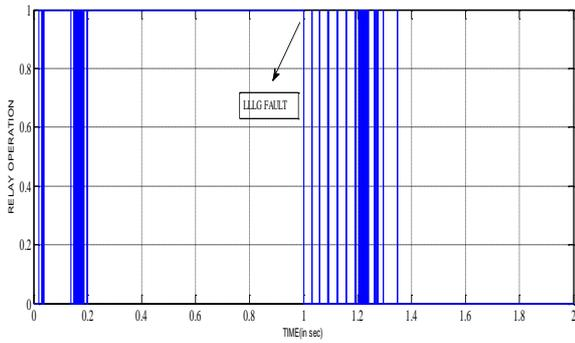
**Figure 18.** Plot of Relay operation during three phases to ground fault condition without OST
