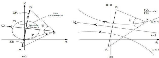
**Figure 5.** (a) & (b) Impedance trajectories at the Relay during a Power Swing for Different  $k$  Values
