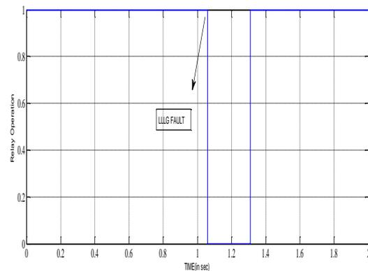
**Figure 14.** Plot of Relay operation during three phases to ground fault condition
