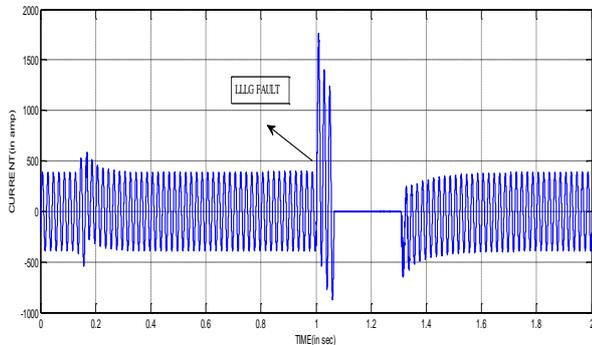
**Figure 15.** Plot of Current during three phases to ground fault condition
