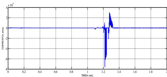
**Figure 19.** Plot of Current during three phases to ground fault condition without OST
