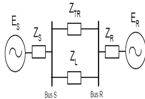
**Figure 8.** Two-Source System Equivalent
