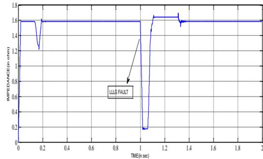
**Figure 13.** Plot of impedance during three phases to ground fault condition
