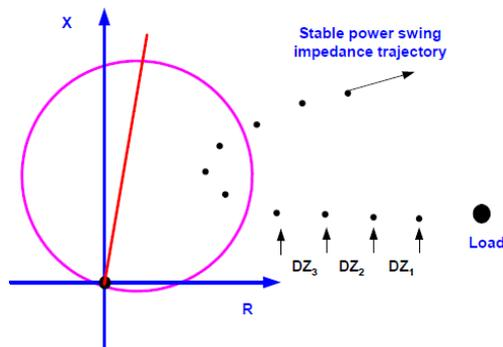
**Figure 7.** Power swing detection with continuous impedance calculation
