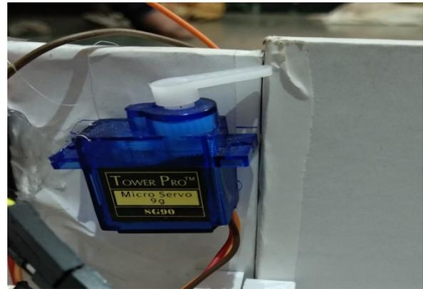
Figure 5. Door lock servomechanism
