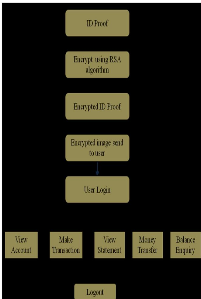
**Figure 3.** Block Diagram of proposed System
