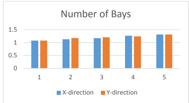
Variation of Redundancy factor with no of bays
