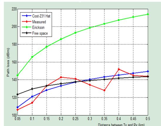
**Figure 3:** Path loss against distance at 6m receiver height.
