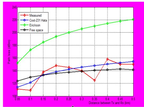
**Figure 1 :** Path loss against distance at 2m receiver height
