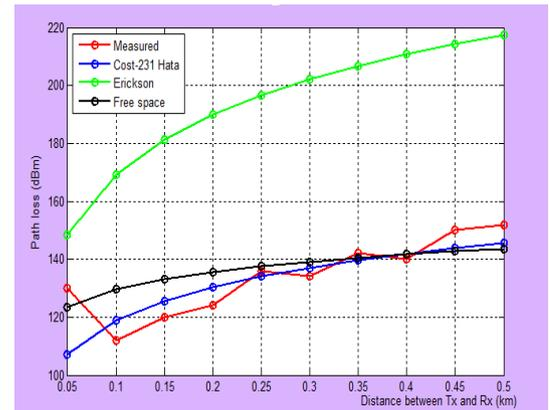
**Figure 2 :** Path loss against distance at 4m receiver height.
