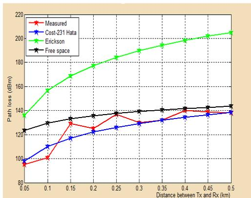
Figure 5 : Path loss against distance at 10m receiver height.
