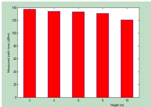
Figure 6 : Measured mean path loss against height
