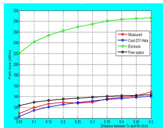
**Figure 4 :** Path loss against distance at 8m receiver height.
