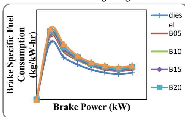
Figure 2. Variation of brake specific fuel consumption with power output
