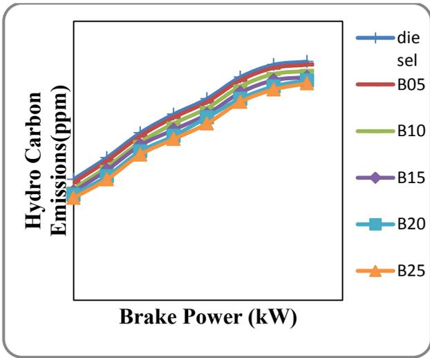
Figure 5. variations of hydrocarbon emissions with power output
