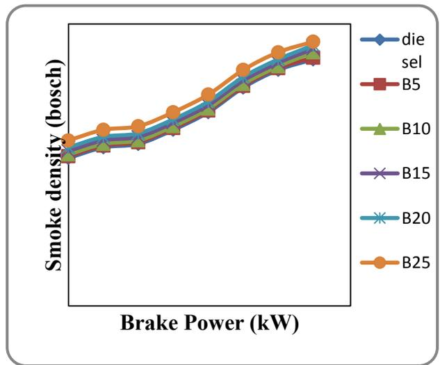
**Figure 4.** Variation of smoke density with power output
