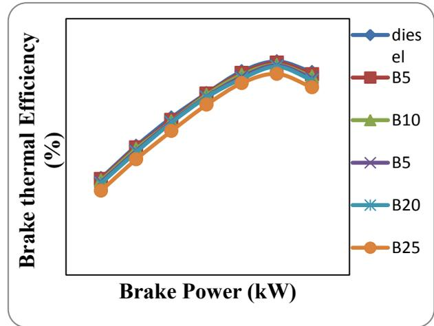
Figure 1. Variation of Brake thermal Efficiency with power output
