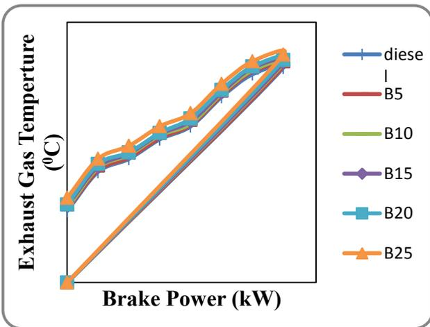
Figure 3. Variation of Exhaust gas temperatures with power output
