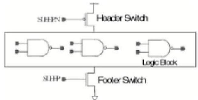
Figure 2: MTCMOS Circuit
