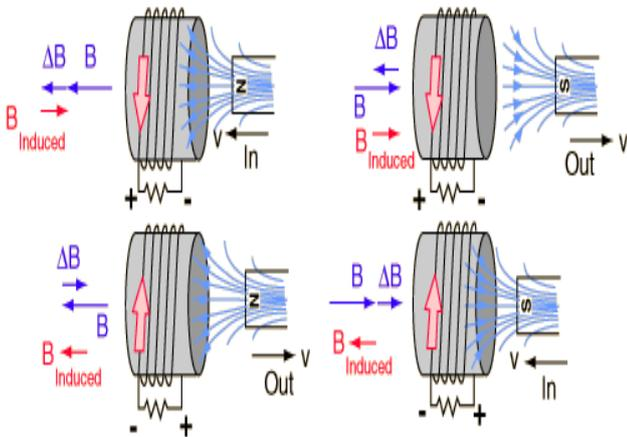
Figure 2. Magnetic flux changes
