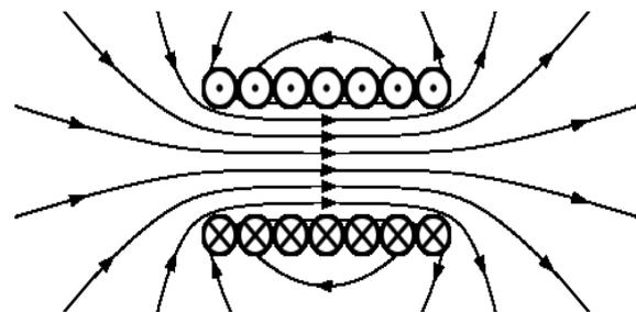
Figure 1. magnetic field produced by a coil of wire
