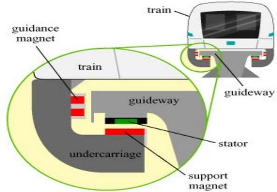
Figure 4. Magnetic levitation trains
