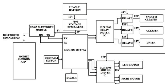
**Figure 3.** Block Diagram of Smart Floor Cleaner
