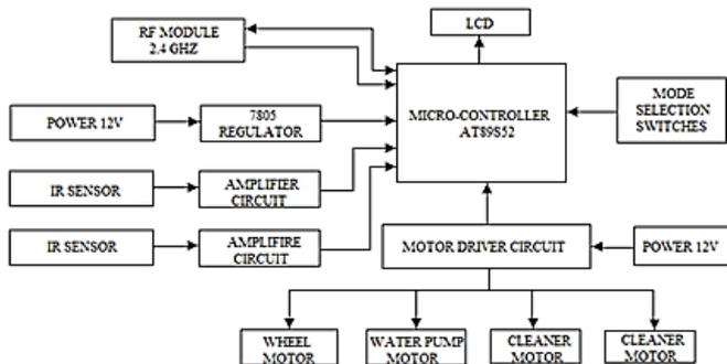
**Figure 2.** Block Diagram of Wireless Floor Cleaning Robot
