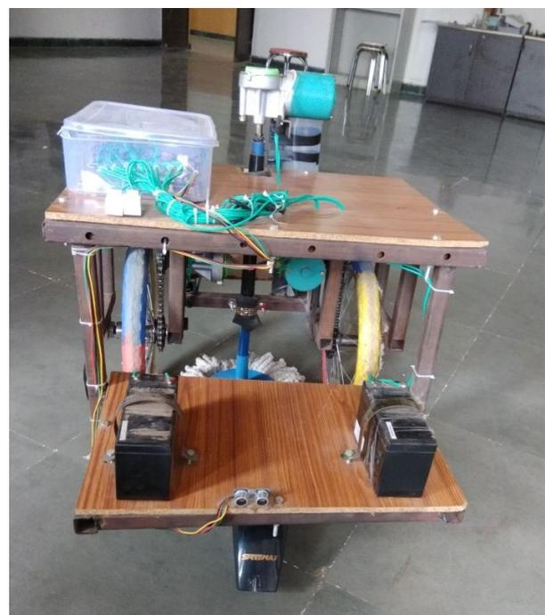
**Figure 6.** Hardware Model of Smart Floor Cleaner
