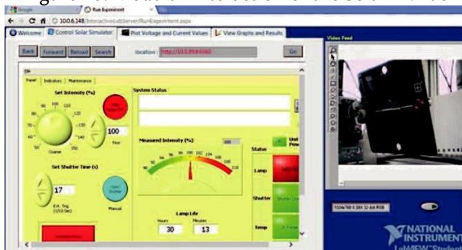
Figure 11: The Control Solar Simulator Tab
