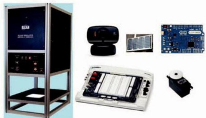
Figure 1: Left: Solar Simulator Top Left: c170 Logitech webcam, solar panel, Arduino Leonard board Bottom Left: NI ELVIS 11+, Servo Motor
