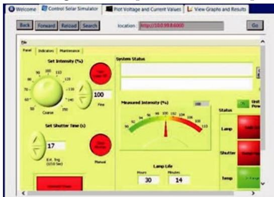
Figure 2: Remote control of the solar simulator using LabVIEW
