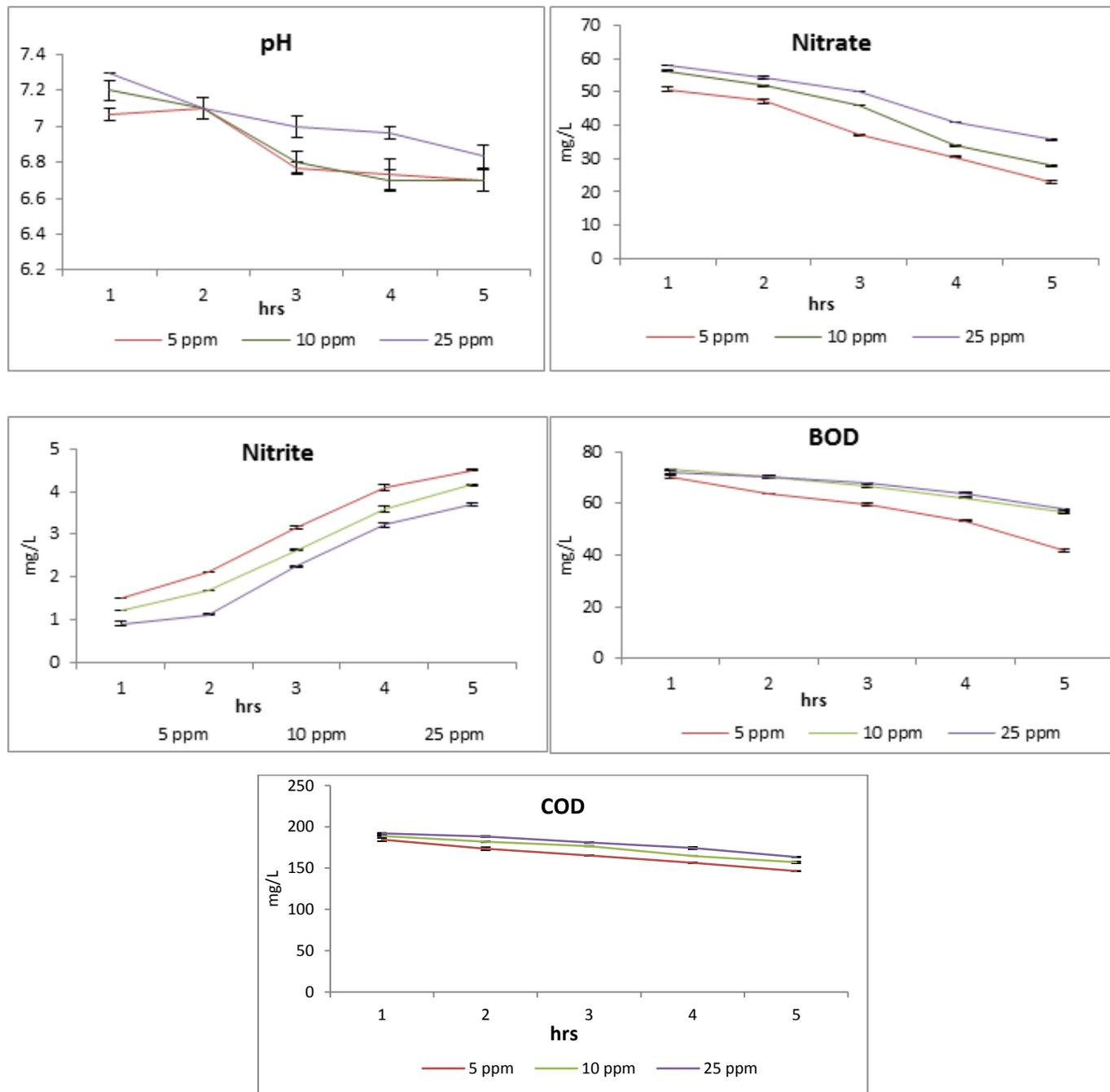
**Figure 4:** Variation of environmental conditions during bioremediation (\*\*Data presented are the mean of triplicates with standard error (5%))
