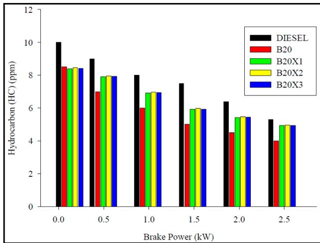
**Figure 10:** Variations in Hydrocarbon Emission with Brake Power and different Additives using B20 Fuel
