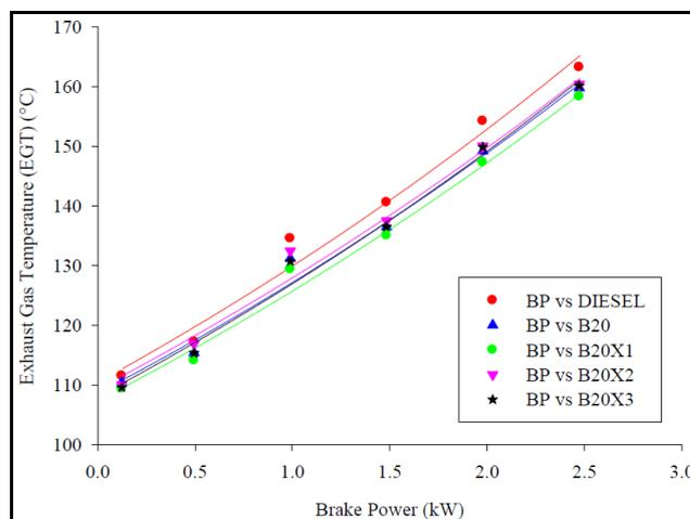
**Figure 6:** Variations in Exhaust Gas Temperature with Brake Power and Different Additives using B20 Fuel
