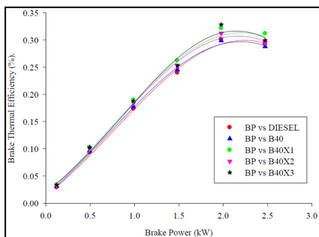
Figure 3: Variations in Brake Thermal Efficiency with Brake Power and different Additives using B40 Fuel
