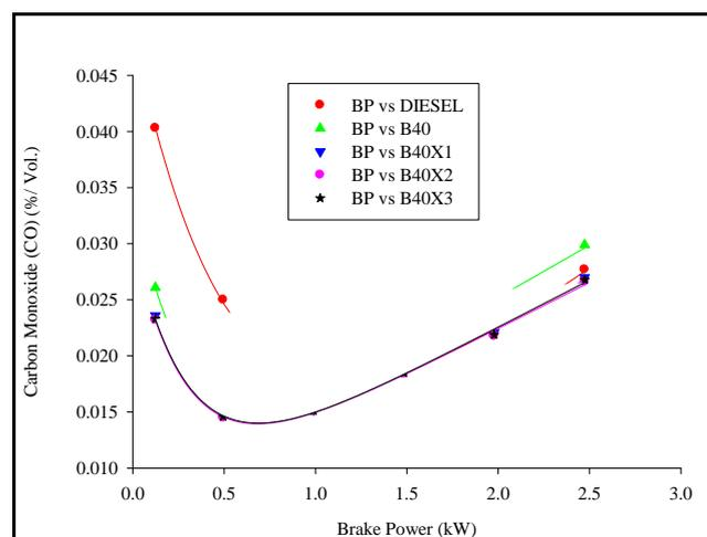
**Figure 9:** Variations in Carbon Monoxide Emission with Brake Power and different Additives using B40 Fuel
