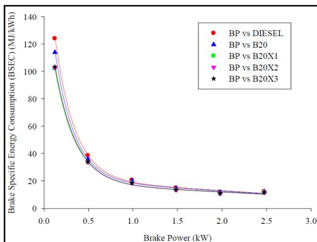
**Figure 4:** Variations in Brake Specific Energy Consumption with Brake Power And different Additives using B20 Fuel
