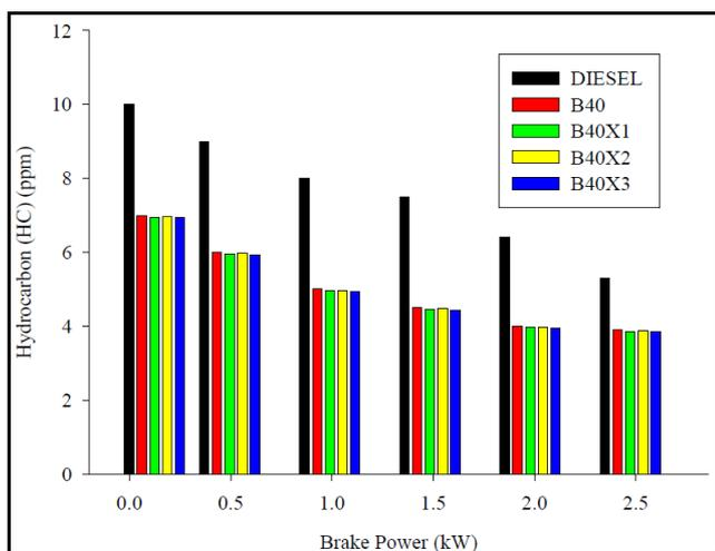
**Figure 11:** Variations in Hydrocarbon Emission with Brake Power and different Additives using B40 Fuel
