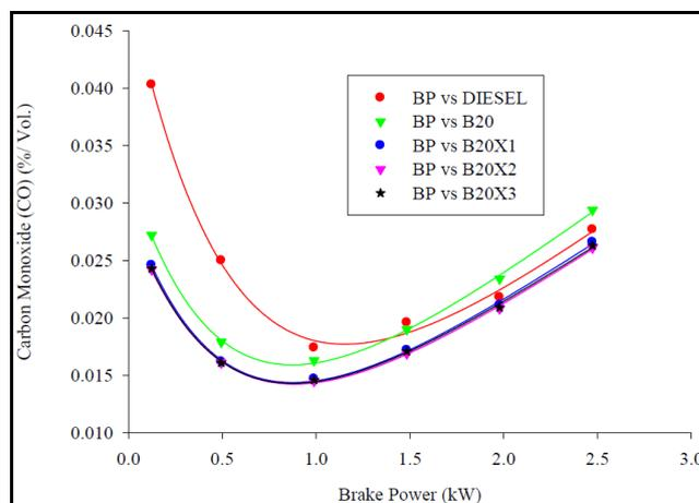
**Figure 8:** Variations in Carbon Monoxide Emission with Brake Power and different Additives using B20 Fuel
