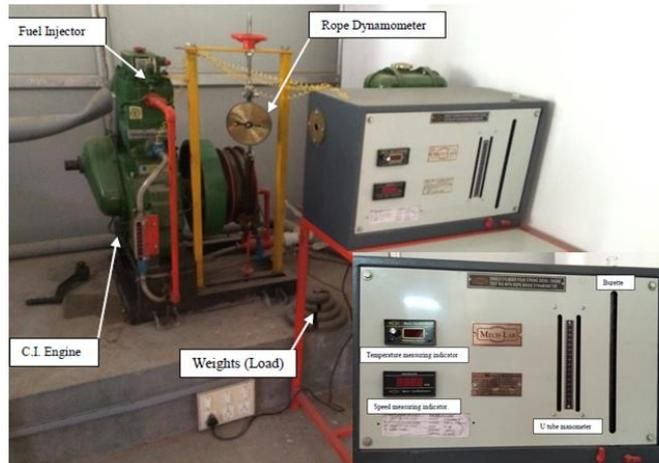
Figure 1: Engines with Control Panel
