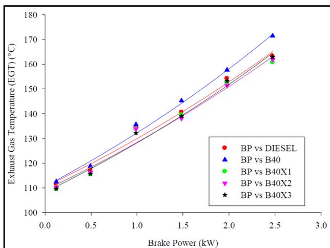
**Figure 7:** Variations in Exhaust Gas Temperature with Brake Power and Different Additives using B40 Fuel
