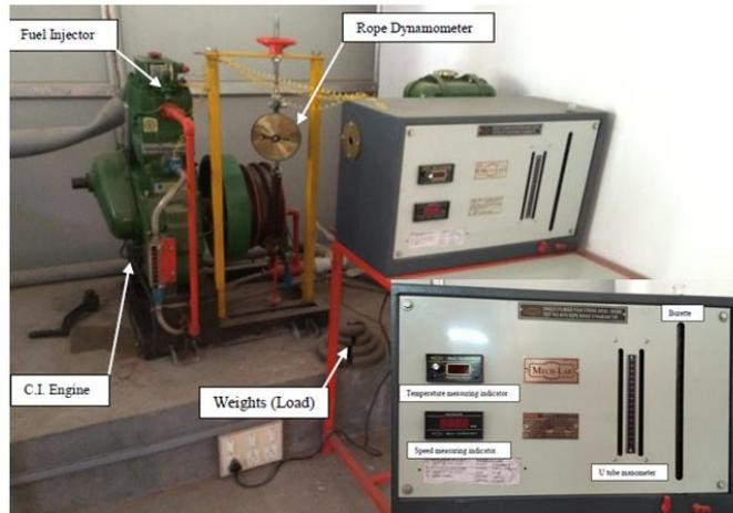
Figure 1: Engines with Control Panel
