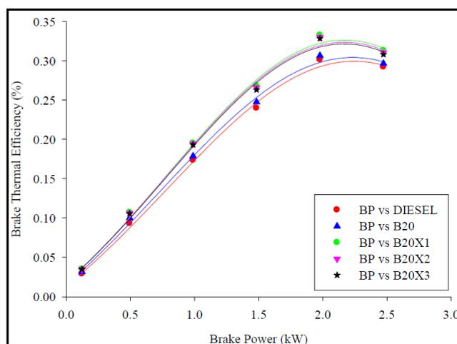
Figure 2: Variations in Brake Thermal Efficiency with Brake Power and different Additives using B20 Fuel
