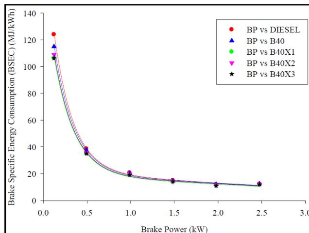
**Figure 5:** Variations in Brake Specific Energy Consumption with Brake Power And different Additives using B40 Fuel
