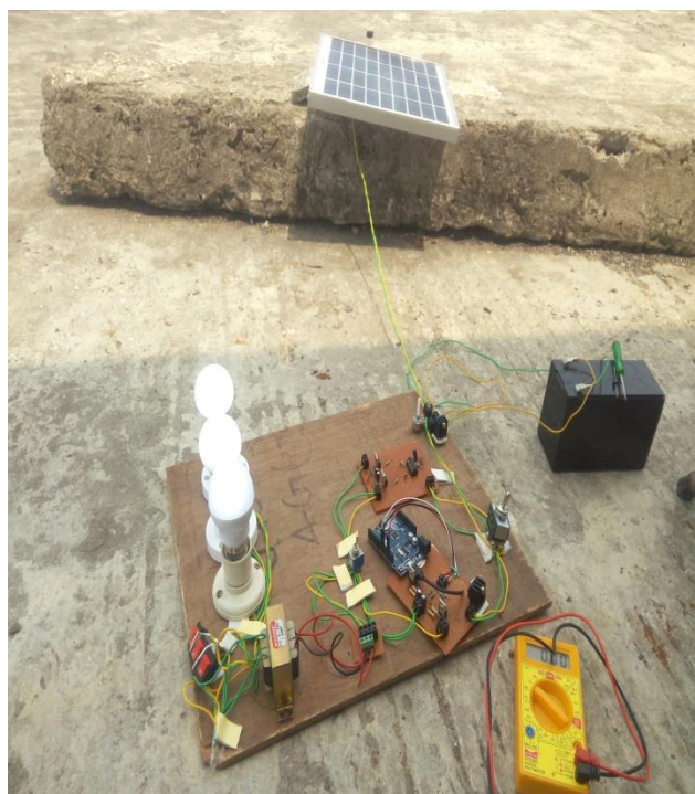
Figure 8 : Complete inverter kit
