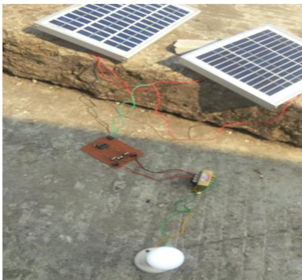
Figure 4(ii): output of IC based inverter with using Solar panel
