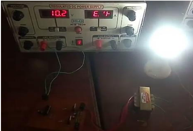
Figure 4(i): output of IC based inverter with using RPS
