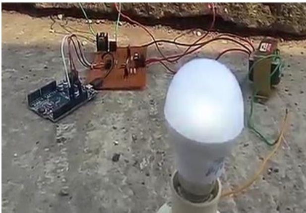
Figure 7(ii): Output of ARDUINO based inverter with using Solar panel
