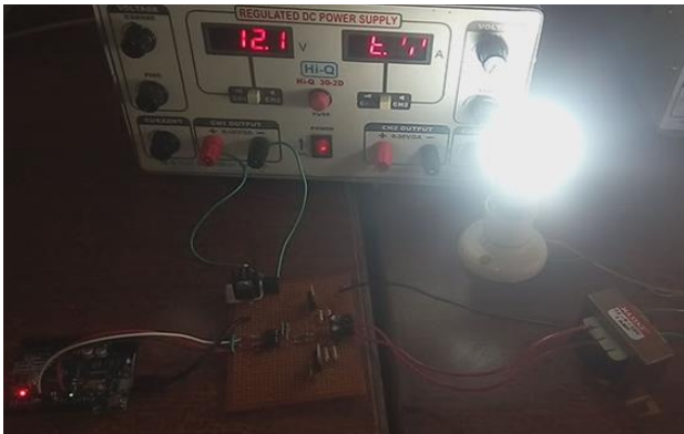
Figure 7(i): Output of ARDUINO based inverter with using RPS
