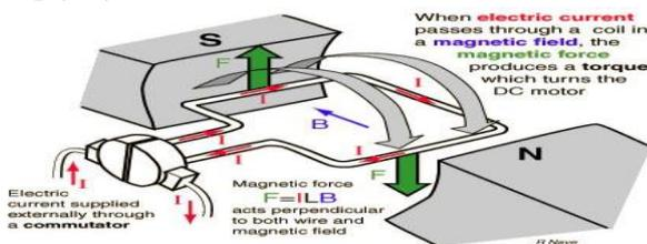
Figure 5.1. DC motor mechanism adapted from NCERT
