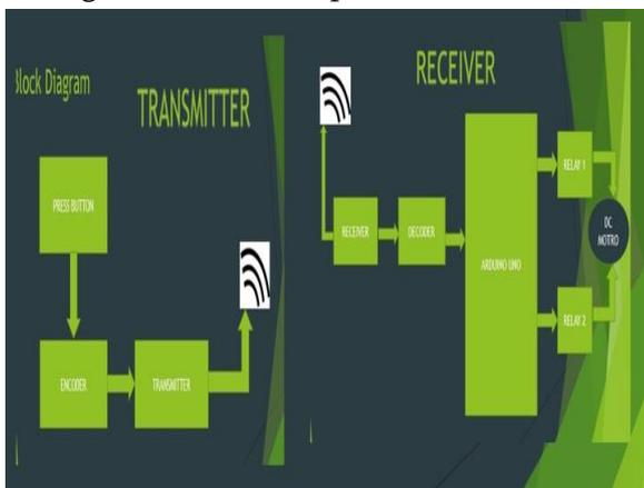
Figure 3.1. Block diagram
