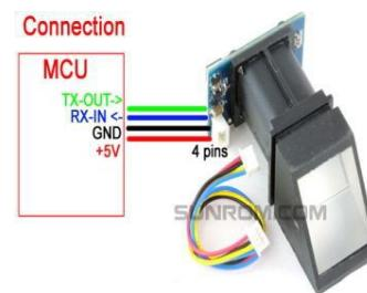
Figure 4. Fingerprint module
