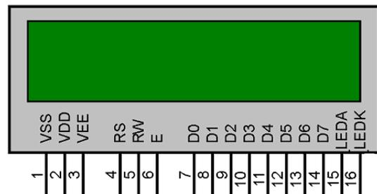
Figure 5. Liquid Crystal Display
