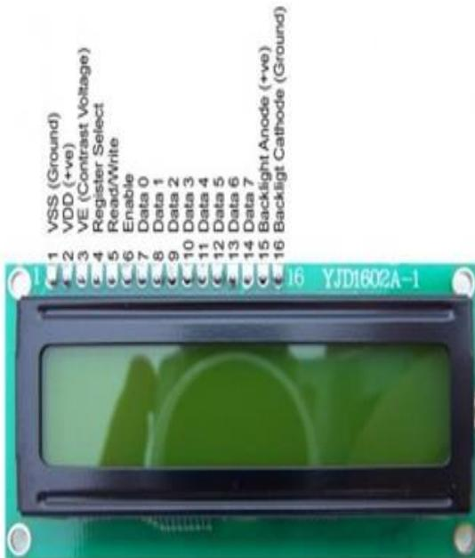
Fig.6 Lcd Display
