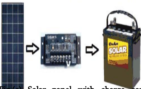
Fig.(c) Solar panel with charge controller and battery
