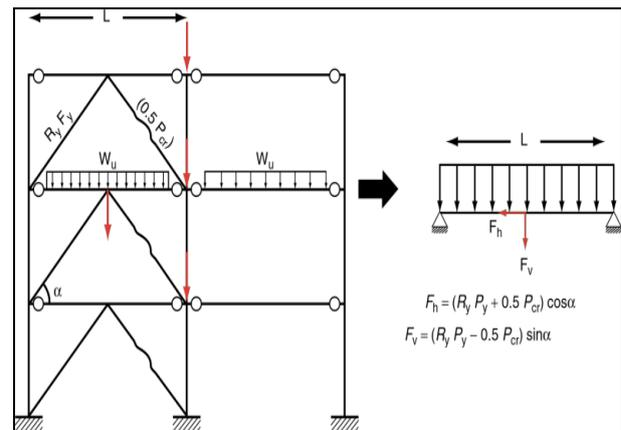
Figure 1. Beam Design Forces for a Chevron Type CBF Axial Load:
