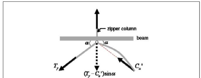
Figure 4 Post-buckling vertical unbalance force (Jeongjae Kim et al. (2008) )
