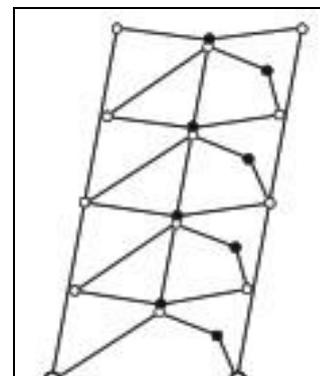
Figure 5 Full height Collapse mechanism of Zipper frame
