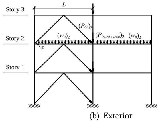
Figure 2 (a & b) Axial force components for brace pre-buckling limit state
