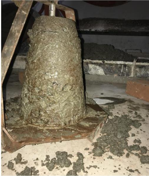
Figure 4: Slump test
