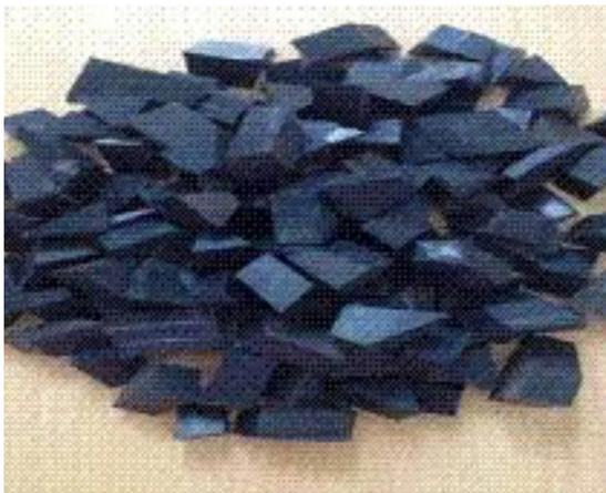
Figure 1: Rubber aggregate
