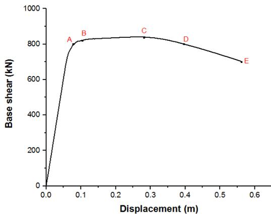
Fig 9 Performance point on capacity curve
