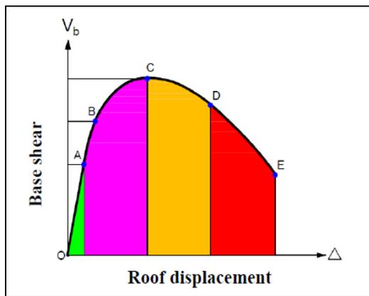
Fig. 1 Damage index estimation methods critical points
