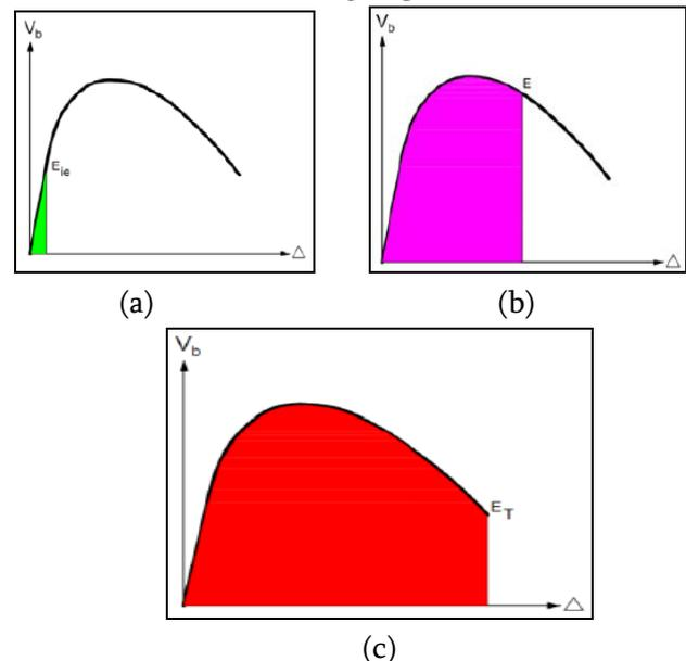
Fig. 2 Damage estimation parameter for Method-1 Where  $E$  – Represents the energy dissipated at any displacement by the structure, where the damage is to be estimated.
