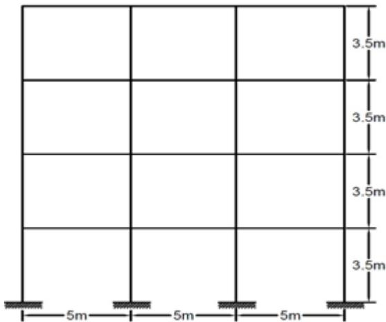
Fig. 6 Elevation of 4 storey RC frame
