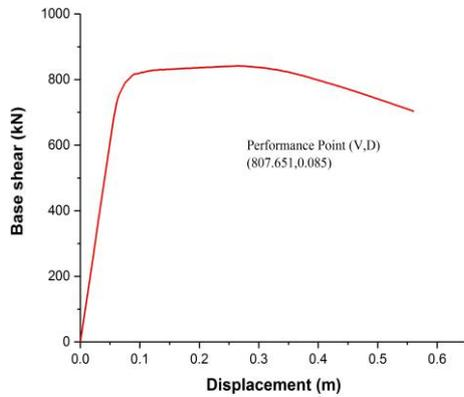
Fig 8 Capacity curve for 4 storey RC frame
