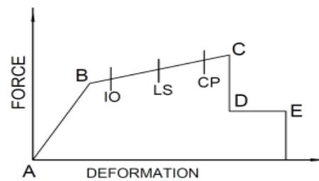
Fig 7 Generalized force deformation curve
