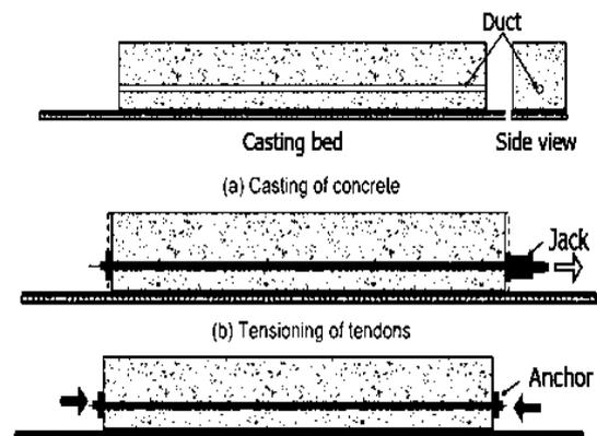
Most of the commercially patented prestressing systems are based on the following principle of anchoring the tendons:
