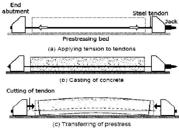
The various methods by which pre-compression are imparted to concrete are classified as follows:
