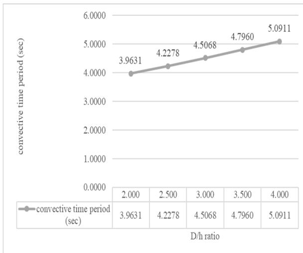
Fig. 2 convective time period vs D/h ratio
