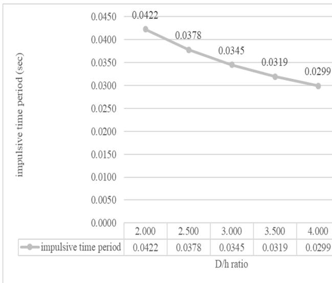
Fig.4 impulsive time period vs D/h ratio
