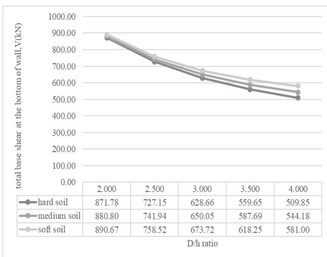
Fig. 3 total base shear vs D/h ratio
