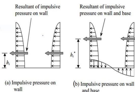
Fig. 2 impulsive and convective hydrodynamic pressure
