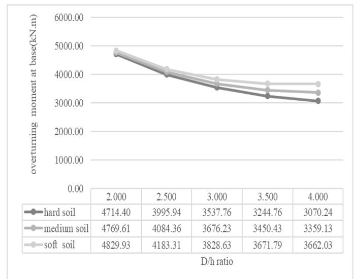
Fig. 5 overturning moment vs D/h ratio
