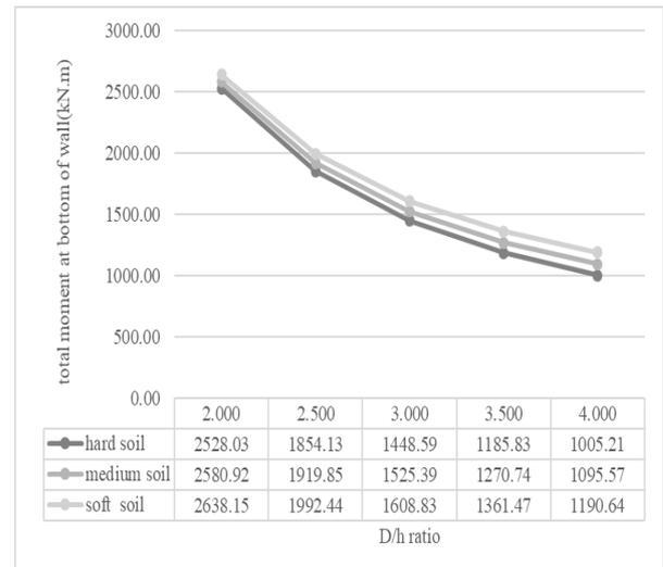
Fig. 4 total moment at bottom of wall vs D/h ratio
