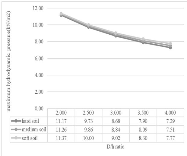
Fig. 7 maximum hydrodynamic pressure vs D/h ratio
