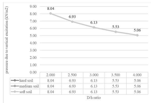
Fig. 6 pressure due to vertical excitation vs D/h ratio
