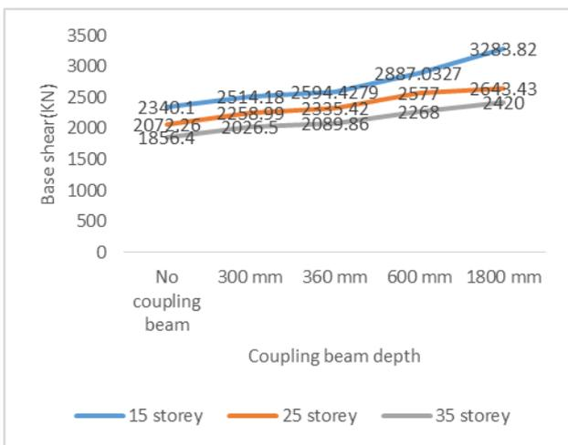
Figure 3: Comparison of Base shear
