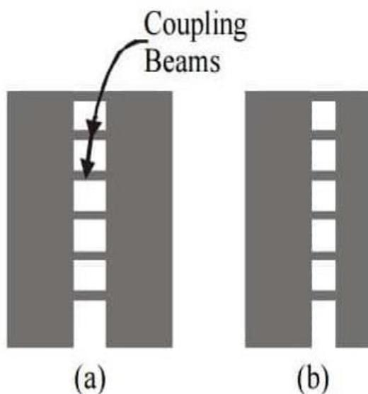
Figure 1: example of coupling beam in structure
