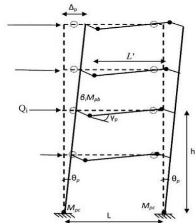
Fig. 2: Pre-Selected Yield Mechanism of Moment Frame with Beam Plastic Hinges away from Column Faces
