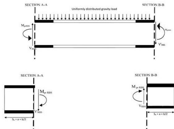
Fig. 4: Free-Body Diagram between Centre of RBS and Face of Column
