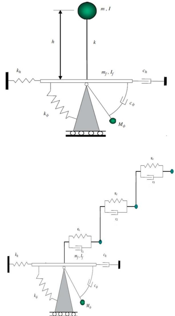
Fig. 1: Soil structure model for sway and rocking motion for SDOF and MDOF systems.
