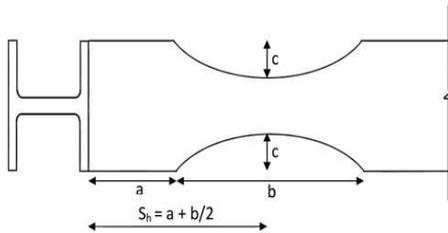
Fig. 3: Reduced Beam Section
