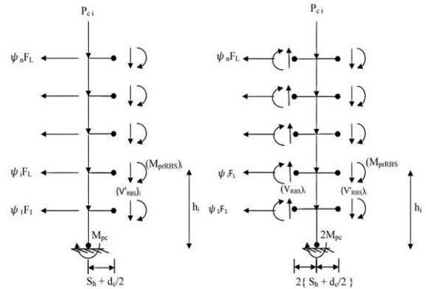
Fig.5: Free-body Diagram of Exterior Column Tree and Interior Column Tree
