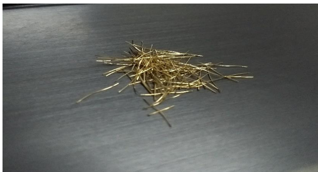
Figure 1: Brass Coated Micro Steel Fibre (13 mm)
