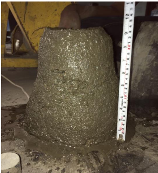
Figure 3: Slump of Geo-polymer concrete
