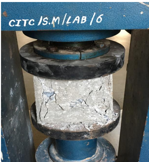
Figure 4: Failure of cube specimen in compressive strength
