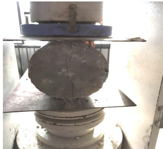
Figure 6: Failure of cylinder in split tensile strength
