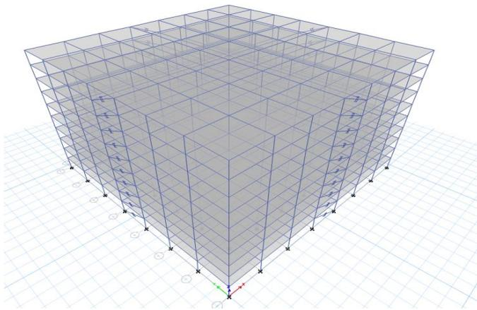
Fig3: 3D view of 10 story building with damper
