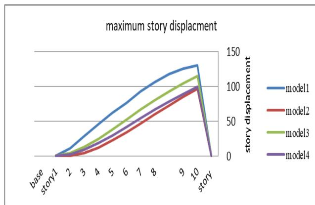
Fig4: maximum story displacement of model buildings.
