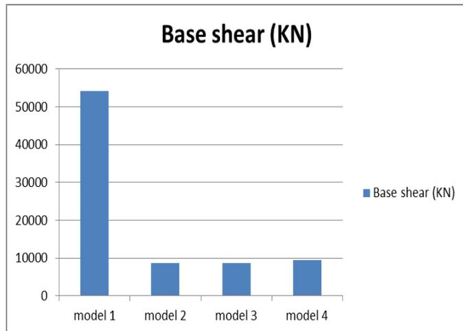
Fig6: base shear for 10 storey model buildings.
