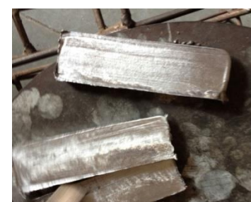
Figure 7: Preparation of Work Pieces through Stir Casting
