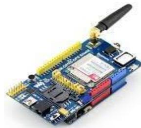
Figure 1. GPS and GSM Module
