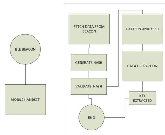
Figure 1: A workflow of how the beacon data is processed inside the mobile application.
