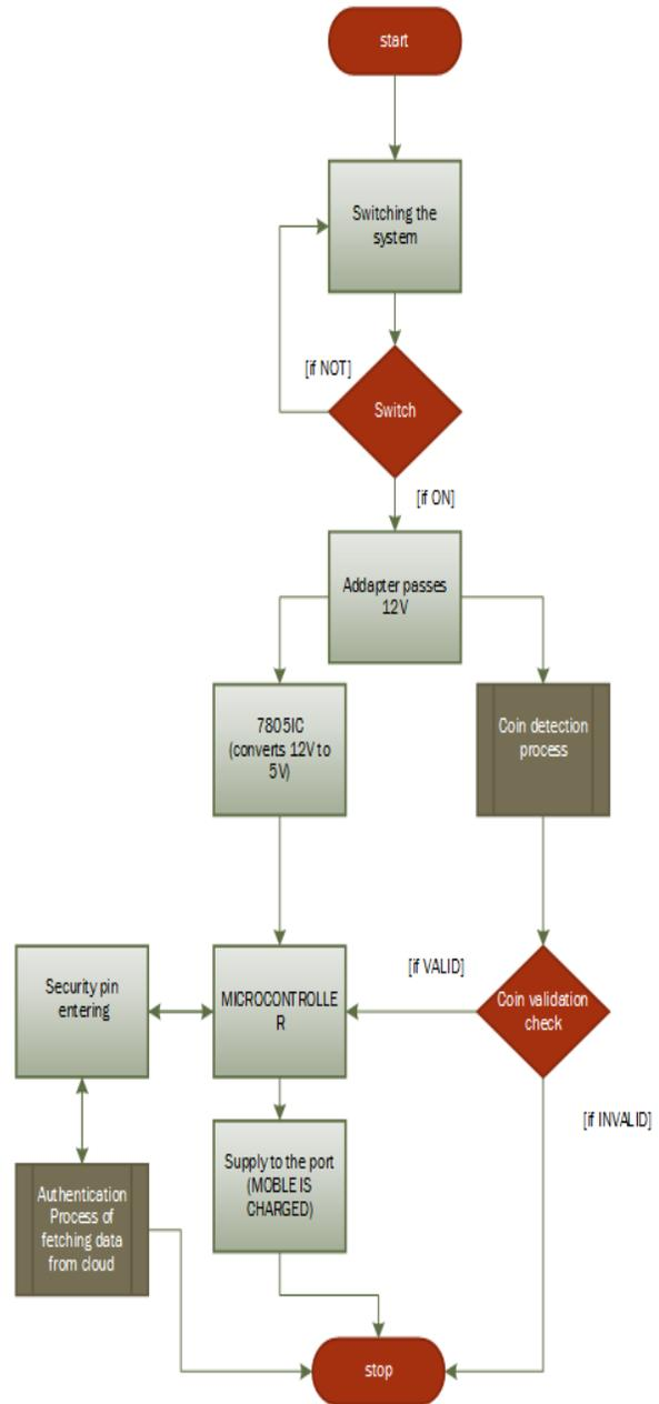
Figure1: Flow diagram of coin based mobile charging system
