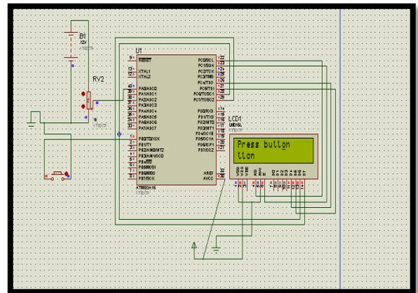
**Figure4:** Here the LCD displays the message to press a button so that the charging circuit can get on.
