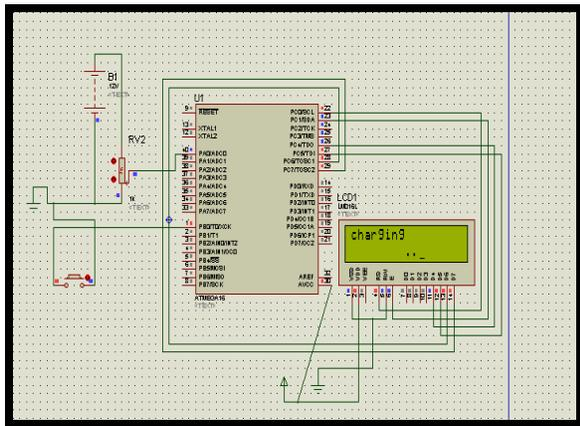
**Figure5:** The button was pressed and the charging circuit is on and the charging gets started. It displays the message that it is charging.
