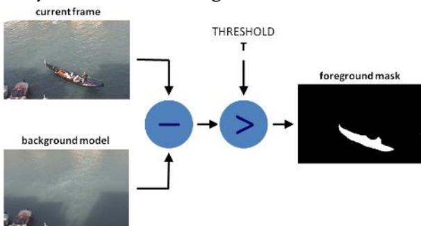
Figure 5: Background Subtraction Model
