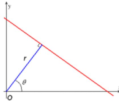
**Figure7:** Hough Transform
