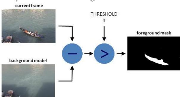
Figure 5: Background Subtraction Model
