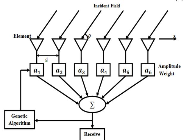
**Figure 1.** Linear half Dipole Array Antenna geometry
