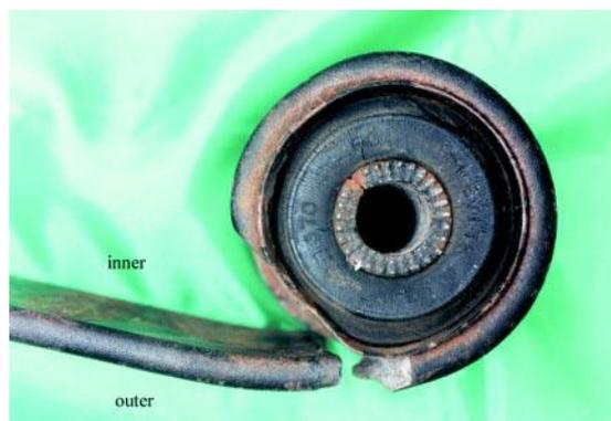
**Fig. 2** The broken halves of the spring have been placed together in a manner exaggerating the opening of the eye before rupture<sup>(3)</sup>
