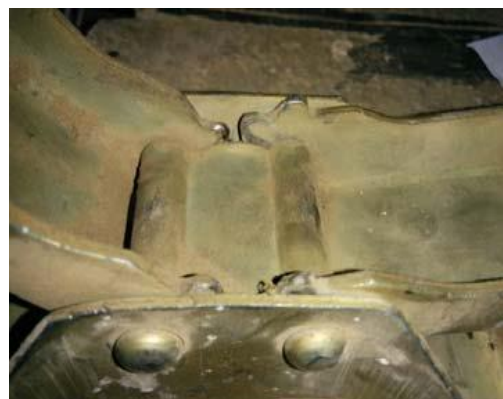
Figure 1 Fig. Teeth Wear of Lower Arm [1]
