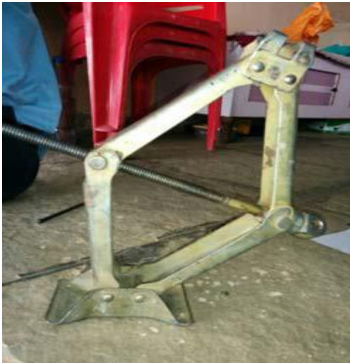
Figure 3 Fig. Topped Scissor Jack due to Arm teeth [3]
