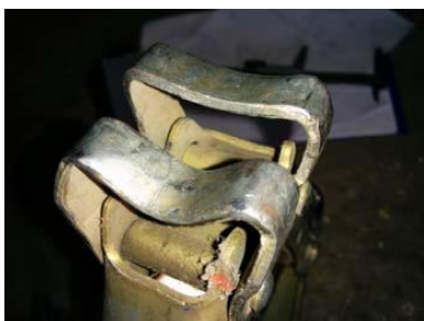
Figure 4 Failure of Jack Head [2]
