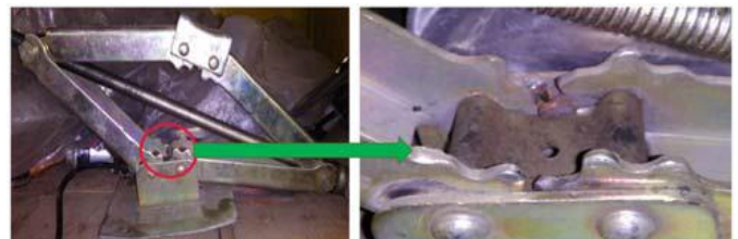
Figure 2 Fig. Failure of Screw and Arm Teeth [2]
