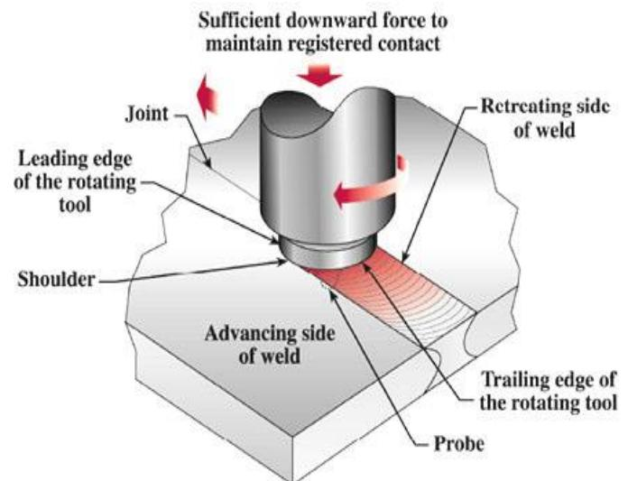
Friction stir welding principle [8]
