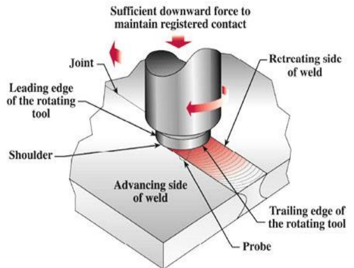
Friction stir welding principle [8]
