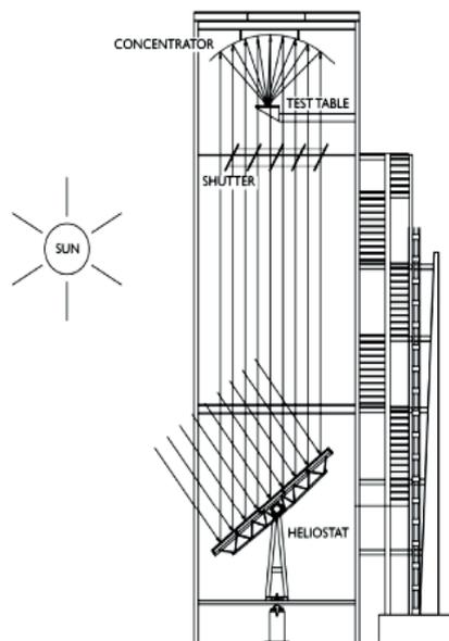
Figure 1 Vertical axis solar furnace<sup>[1]</sup>
