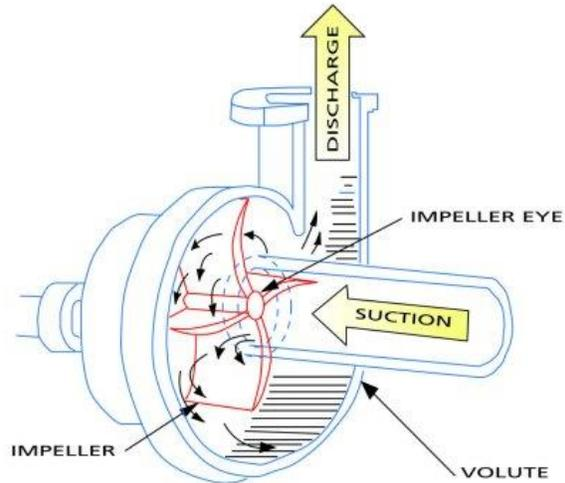
Figure 1 – Centrifugal Pump
