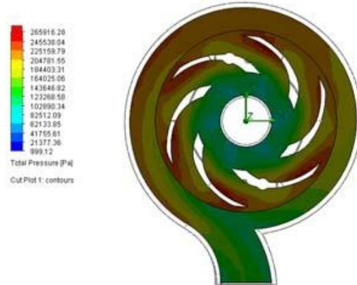
Figure 2 – Design & analysis of pump impeller
