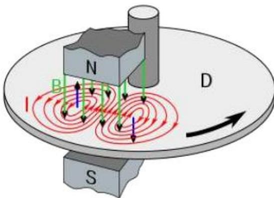
Fig. 1: Braking system using eddy current
