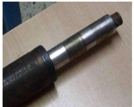
Figure 1.1 Worm out bearing surface of the rotor
