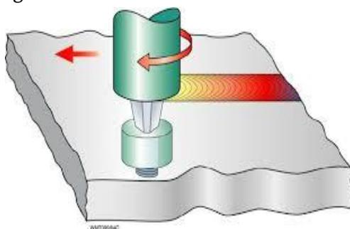
Figure 2: Schematic of Bobbin Tool [1]
