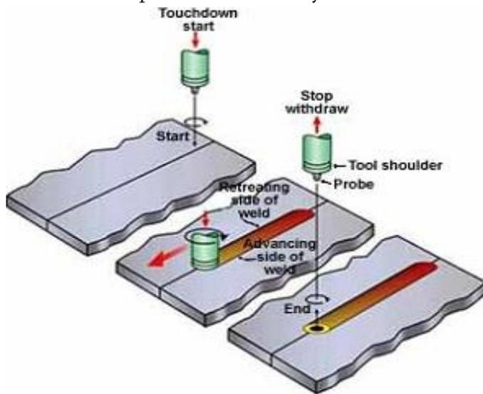
Fig-1 friction stir welding principle [2]
