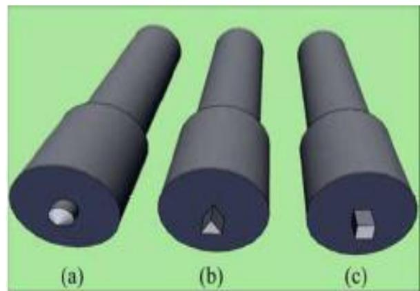
Figure 5 Tool pin geometries: (a) Threaded tapered cylindrical pin (b) Triangular pin (c) Square pin [7]
