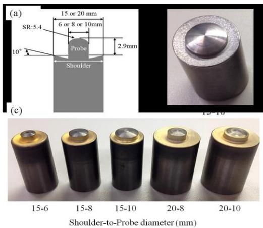
Figure 4 Shoulder to probe diameter [5]
