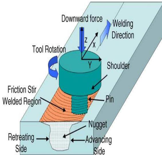
Figure 1 Principle of friction stir welding<sup>[1]</sup>
