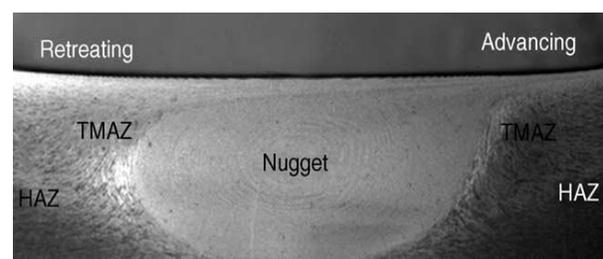
Figure 2 Microstructure of FSW Welded joint<sup>[2]</sup>
