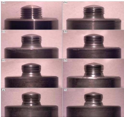
Figure 3 Appearance of threaded tool after each FSW experiment [4]
