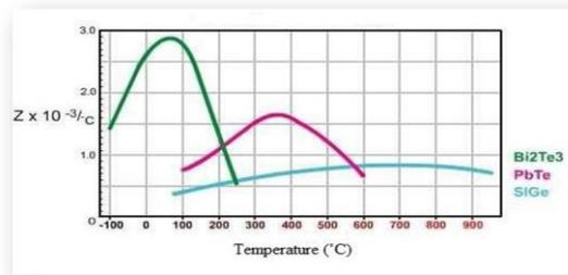
**Figure6:** Performance of Thermoelectric Materials at various temperatures
