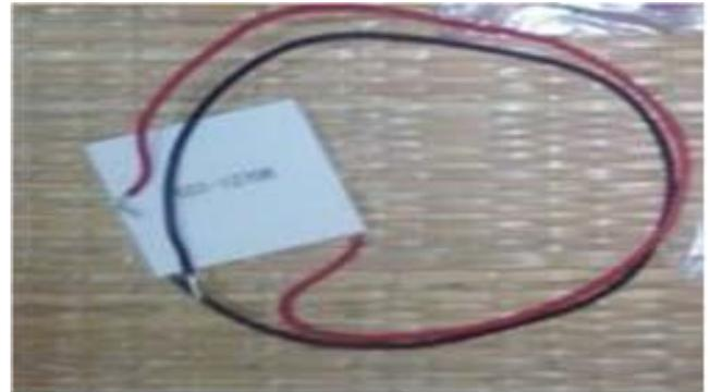
Figure 2: Peltier Module
