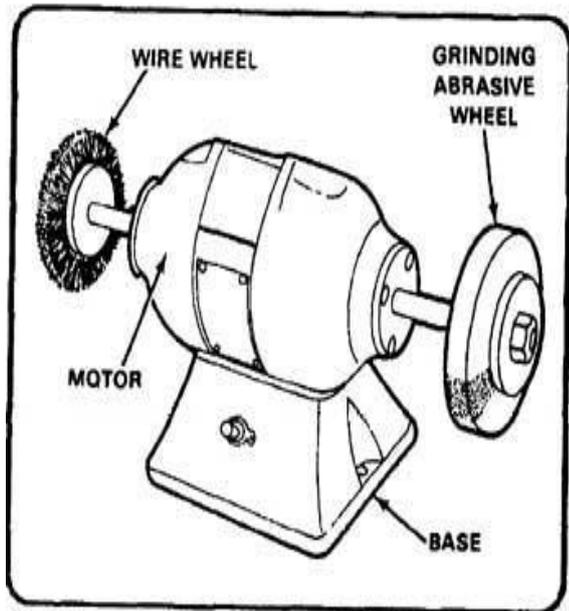
Fig:1.2 Grinding Machine
