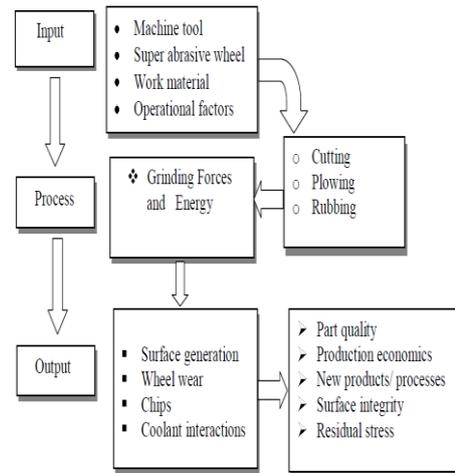
Fig :2.1 Working Principle of Grinding
