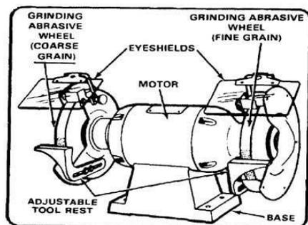
Fig:1.1 Grinding Machine
