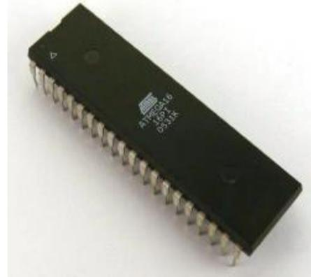
**Figure 3:** Microcontroller ATMEGA16
