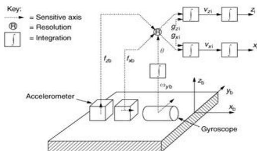
Figure 1: Strap-down inertial navigation system.[11]
