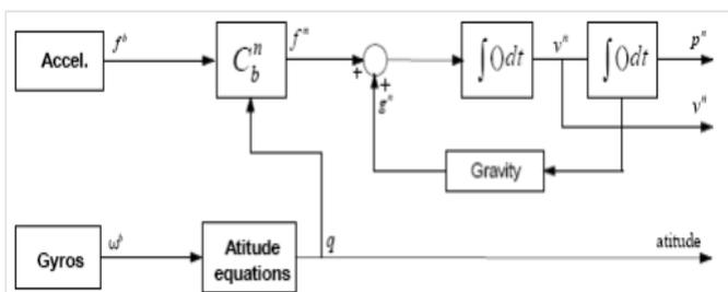
Figure 4: IN mechanization diagram - Navigation frame
