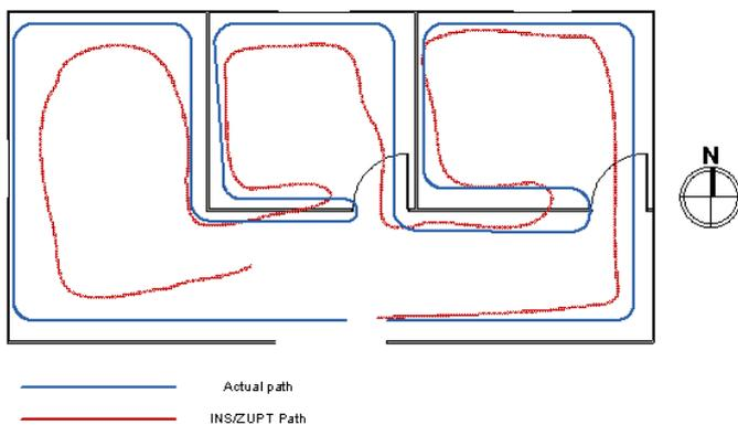
(Fig. 14) this figure shows how the INS/ZUPT Path (red) followed the actual path (blue) at indoor environment
