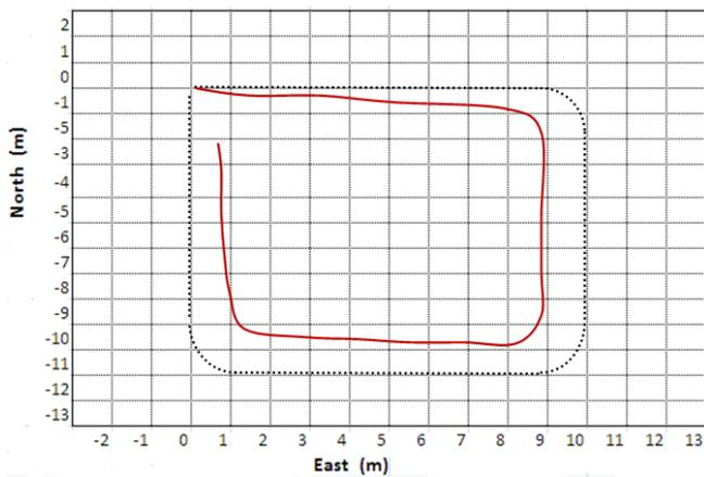
(Fig. 13) The path of INS using ZUPT method
