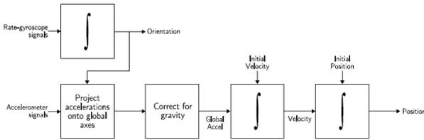
Figure 3: Strap-down inertial navigation algorithm.[10]
