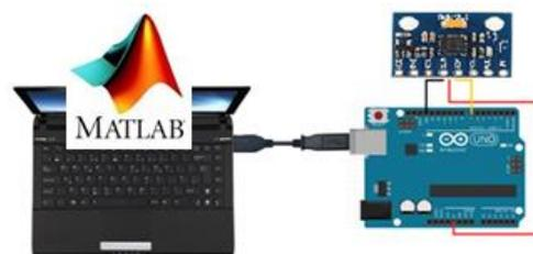
**Figure 10:** Hardware Configuration
