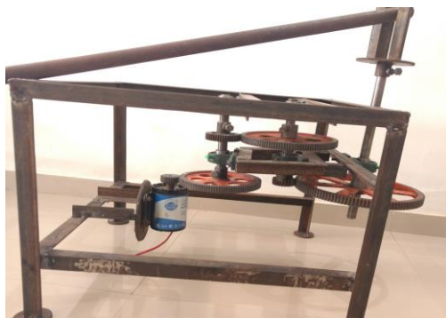
Figure 2: A sample assembly for power generation
