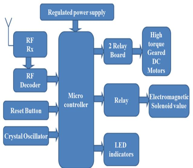
Figure 4.3 block diagram of receiver
