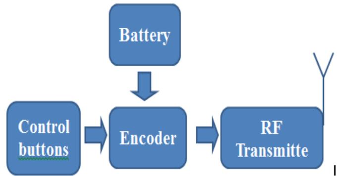
Figure 4.2 Block diagram of transmitter
