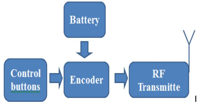
Figure 4.2 Block diagram of transmitter
